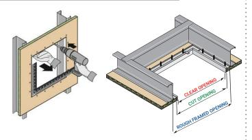
2. The structure surrounding the installed access panel must be rigid. Use blocking/cross members so no framing is more than 4" from the panel opening.
